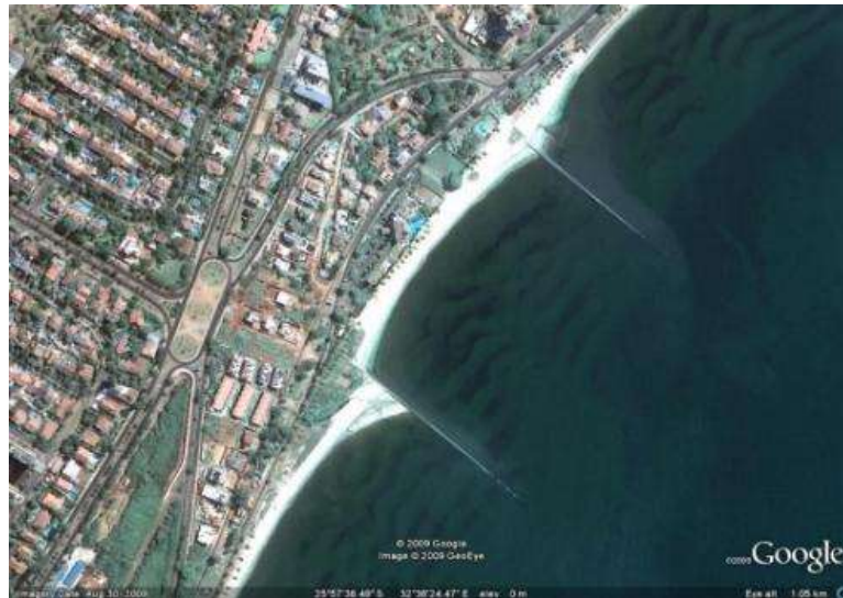
Figure 7.11: Existing groynes along Maputo shoreline
